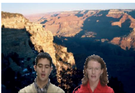
Figure 5. Two arbitrary shaped foreground objects with a JPEG background. Streamed from a server to a client over an IP test bed in our lab.
